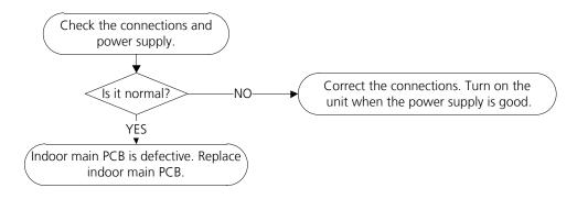
Note: E2/EH 02 zero crossing detection error is only valid for the unit with AC fan motor, for other models, this error is invalid.
