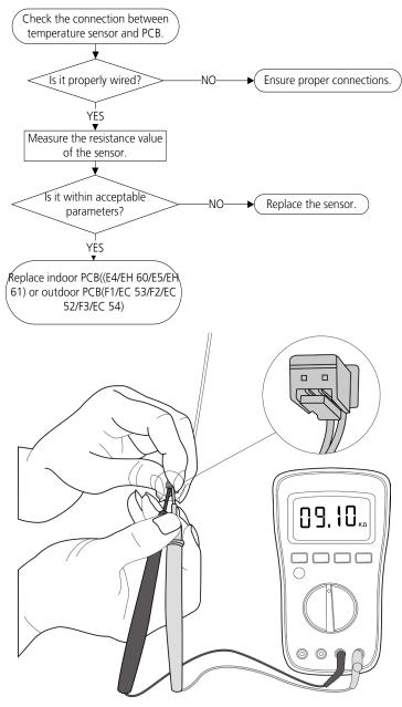
Note: For certain models, outdoor PCB could not be removed separately. In this case, the outdoor electric control box should be replaced as a whole. This picture and the value are only for reference, actual appearance and value may vary. For certain models, outdoor unit uses combination sensor, T3,T4 and TP are the same of sensor.
